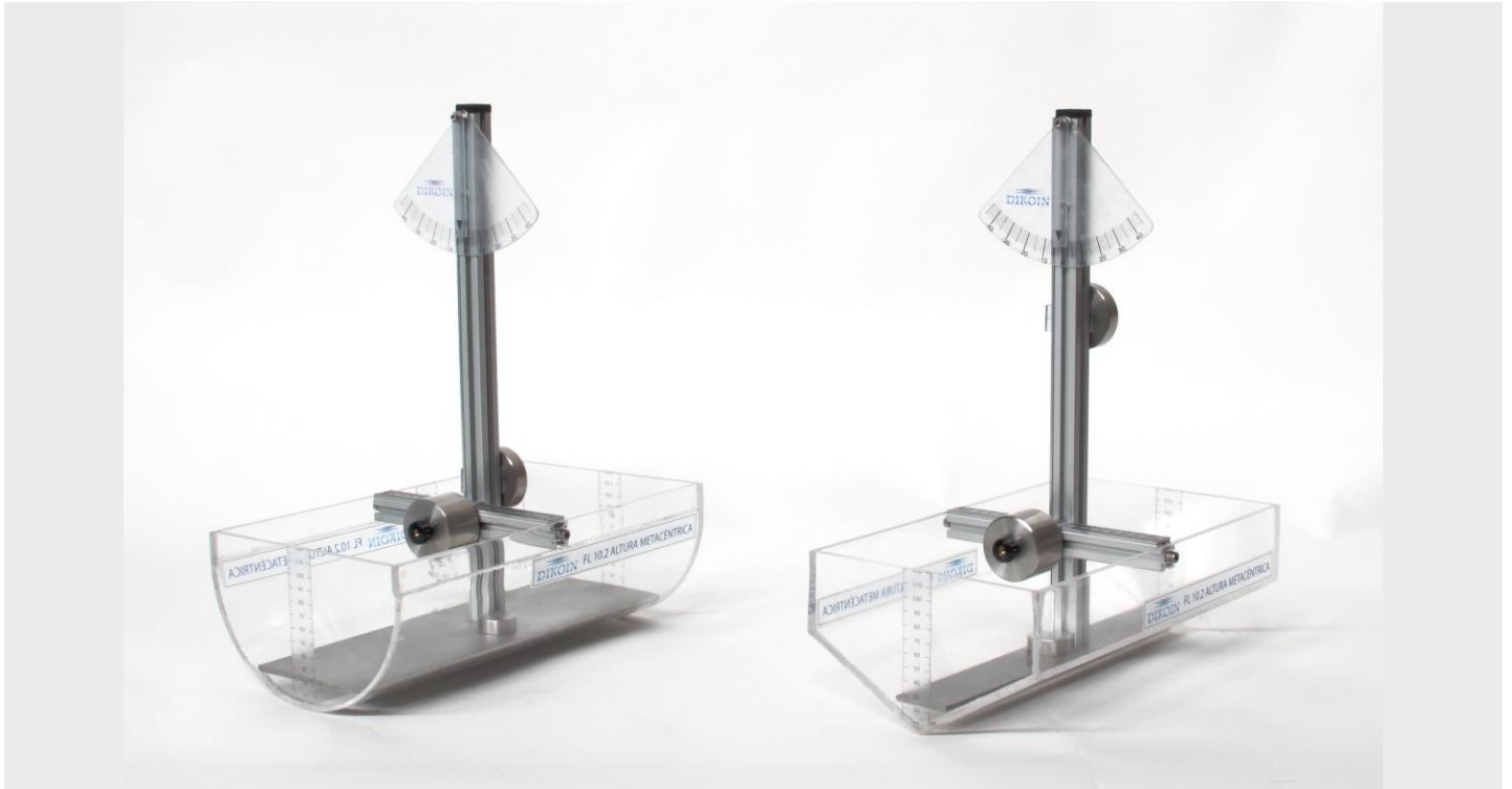
Optional Accessory: FL 10.3 - ADDITIONAL BODIES FOR STUDY OF METACENTRIC HEIGHT 2 Floating bodies with weights and scales for metacentric height calculation. Forms V and U.
